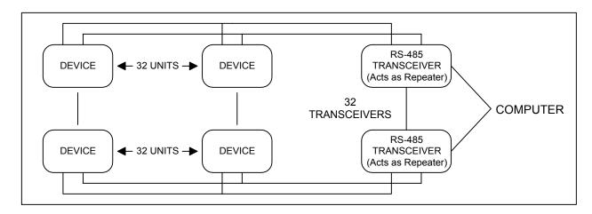
Figure 4.7: 2-Wire RS-485 Communication Installation Connection with Transceiver
